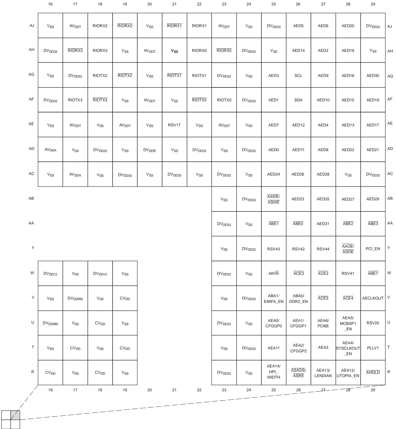
Figure 2-3. C6455 Pin Map (Bottom View) [Quadrant B]
