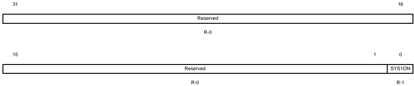
Figure 7-29. SYSCLK Status Register [Hex Address: 029C 0150]
